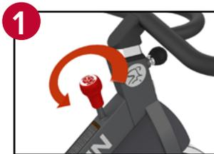
**STEP 1:** Remove tension from the brake pad by turning the resistance knob counterclockwise as far as possible. You should feel a “stop” when the knob is completely loose and you should not rotate the knob any farther.
