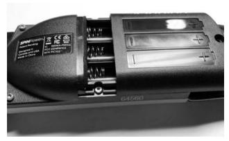
2. Slide the cover forward (towards the pedal side) as shown to reveal the battery compartment. Note the orientation of the 3 AA batteries.
