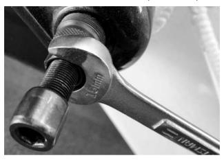
3. Once started by hand, use a wrench and turn it clockwise to thread the tool completely into the crank.
