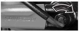
2. Once the crank is on, hand-thread the 8mm bolt clockwise onto the axle. Now use an 8mm torque wrench to tighten the bolt to 35-40 ft-lbs (47-57 Nm).
