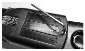
1. Use the 3mm allen wrench to remove the single allen bolt on the battery door (as shown).
