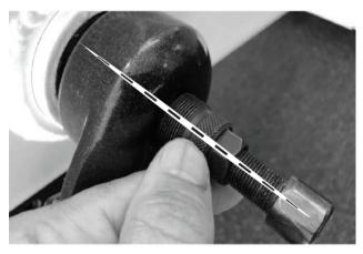
2. The process for removing the crank is exactly like removing the pedal (prevously outlined). Before threading in the crank removal tool, unthread the center bolt (on the tool) so that the tip is recessed (see diagram on page 9). Once set, thread the body of the crank removal tool into the fine threads of the crank. It is VERY IMPORTANT that this tool is threaded into the crank in a straight manner. Do not cross-thread this tool.
