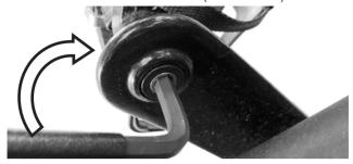
3. Once the crank has been tighened it is time to install the pedal. Locate the 8mm pedal bolt and hand thread it into the pocket on the back of the crank. Now use an 8mm torque wrench and tigthen the bolt to 35-40 ft-lbs (47-57 Nm). Do not overtighten the bolt.
