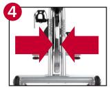
**STEP 4:** While adjusting the chain tension, work equally on both sides of the flywheel. Adjust the angle of the flywheel so that it is straight (front to rear) and evenly spaced within the forks (side to side).
