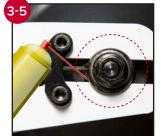
**STEP 6:** Carefully place the chainguard cover back into place and secure it by snugly tightening the screw.
