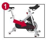
**STEP 1:** Locate the chainguard access panel. Remove the exposed screw
