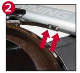
**STEP 2:** Using a wrench, carefully remove the two bolts supporting the brake pad (see red arrows left). Remove the old brake pad assembly.
