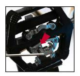
The SPD pedals are set for the lowest release tension at the factory for safety. If you would like a stronger release tension, use a xmm allen wrench and turn the adjustment screw clockwise. Adjust both sides evenly and start with as little adjustment as necessary until you achieve the desired release tension.
