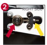
STEP 3: To tighten the chain, use a 10mm box wrench and turn the adjustment screws (see yellow arrow left) in a clockwise rotation equally on both sides
