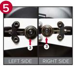
**STEP 5:** Tighten the axle nuts (see red arrow left) on both sides, alternating from side to side until the flywheel is secure.
