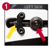
STEP 1: Open the access panel (see Step 1 of chain lubrication process) and local the axle nut.
