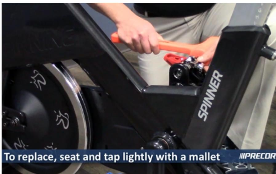
6. Secure pedal with the pedal mounting bolt using an 8 mm hex key, torque to 33 ft-lb (45 N•m).
