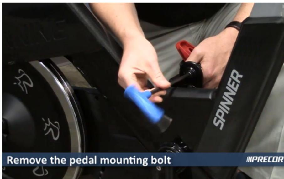
3. Use a crank puller (recommended PN X-Tools Crank Extractor or similar tool) to press the pedal out of the crank arm and remove. Attach the crank extractor to the crank arm
