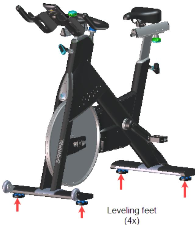
2. Push on the bike and try to rock the bike. If there is any movement make foot adjustments as needed to stabilize the bike. Turn the leveling feet clockwise (+) to lower the bike or counterclockwise (-) to raise the bike.
