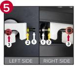
STEP 5: Once the flywheel is centered and the chain is tensioned, check to ensure that the main flywheel adjustment bolts (indicated with white arrows) are touching the flywheel axle. Now tighten the adjustment lock nuts clockwise (indicated with yellow arrows) against the frame while ensuring that the flywheel adjustment bolts do not rotate. Next, tighten the axle nuts (indicated with red arrows) on both sides, alternating from side to side until the flywheel is secure.
