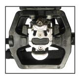
The SPD pedals are set for the lowest release tension at the factory for safety. If you would like a stronger release tension, use a 3mm allen wrench and turn the adjustment screw clockwise. Adjust both sides evenly and start with as little adjustment as necessary until you achieve the desired release tension.
