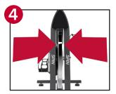
**STEP 4:** While adjusting the chain tension, work on both sides of the flywheel. Adjust the angle of the flywheel so that it is straight (front to rear) and evenly spaced within the forks (side to side).
