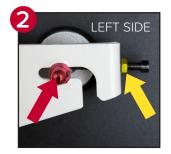
**STEP 3:** To **tighten** the chain, use an allen wrench, to turn the adjustment screws (indicated with white arrows) in a clockwise rotation equally on both sides.
