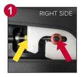
**STEP 1:** To access the axle nut on the right side of the Spinner® bike you will need to first remove the small rubber flywheel adjustment cover. Please refer to Step 2 in the previous section.
