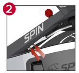
**STEP 2:** Using a 4mm allen wrench, carefully remove the two bolts supporting the brake pad (indicated with red arrows). Remove the old brake pad assembly.
